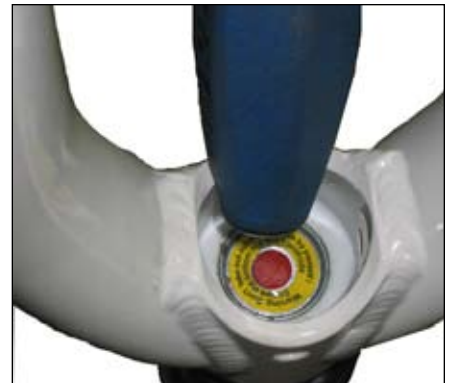
Figure 13. Install red plug
