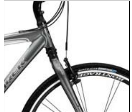
Figure 1. SPA suspension fork, noted by rubber boot above fork crown.
