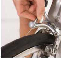
Open up the brake to allow the tire to pass through freely.
