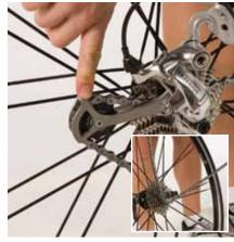
While still holding the frame with your left hand, reach your right hand down to the small tab found on the derailleur above the small wheel. This will cause the chain to slack.
