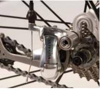
Line up the chain and lay it on the smallest cog of the cassette. Click the dropout into the quick release part of the wheel.
