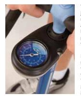
The psi rating range on the side label of mountain bike tires is just that—a range. Most riders over-inflate their tires for off-road mountain bikes out of fear of getting a pinch flat. For most riders a psi setting of 35-40 is fine. However, going too low in psi can lead to side wall cuts much like a tube pinch. So play with psi pressures to find the optimum level that will give you the best traction, control, and protection for the trail you ride on most.
