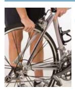
With your left hand, grasp the top tube of the bike and lift the rear wheel off the ground. Since the quick release is open, the wheel will fall out of the dropout.
