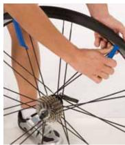
Approximately three inches from the first tire lever, insert the scoop of the second tire lever and pry one side of the tire (also called bead) off the rim.
