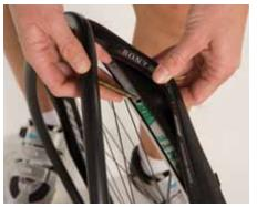
Insert valve stem into the hole in the rim, and feed the tube back into the tire.
