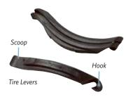
Getting the tire off the rim If the tire is old, you can probably do this with your thumbs. If it's a new tire, or a tight fit, you will probably need tire levers to carefully pry the one side of the tire off the rim.
