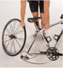
Move the frame away from your body so the chain falls off the rear wheel. Grab the wheel with your right hand and set the bike down on the non-chain side (also known as the non-drive side).
